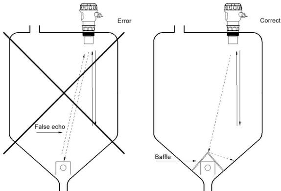
A projection with a flat top at the bottom of the container-a refracting plate should be added.
