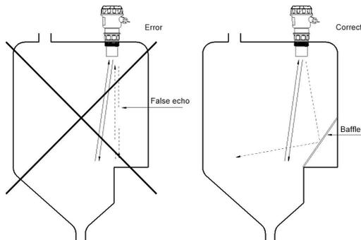
Step-like obstacles in the container-need to add inclined horizontal plates to refract false echoes away
